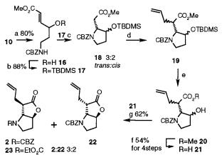
$^a$  (all compounds racemic) (a) CF\_3CO\_2H, CH\_2Cl\_2, 4 °C; (b) tBuMe\_2SiCl, imidazole, DMF, rt; (c) NaH (catalytic), THF, 4 °C; (d) LiN(SiMe\_3)\_2, CH\_2CHCH\_2Br, THF, -78 °C; (e) Bu\_4NF, THF, rt; (f) LiOH, H\_2O, THF, 60 °C; (g) 2,4,6-trichlorobenzoyl chloride, Et\_3N, DMAP, PhMe, reflux.
